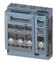
SENTRON, fuse switch disconnector 3NP1, 4-pole, NH1, 250 A, for assembly and installation on mounting plate, Box terminal, cover level 70mm
