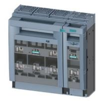
SENTRON, fuse switch disconnector 3NP1, 4-pole, NH2, 400 A, for assembly and installation on mounting plate, Box terminal, cover level  $70 \mathrm{mm}$
